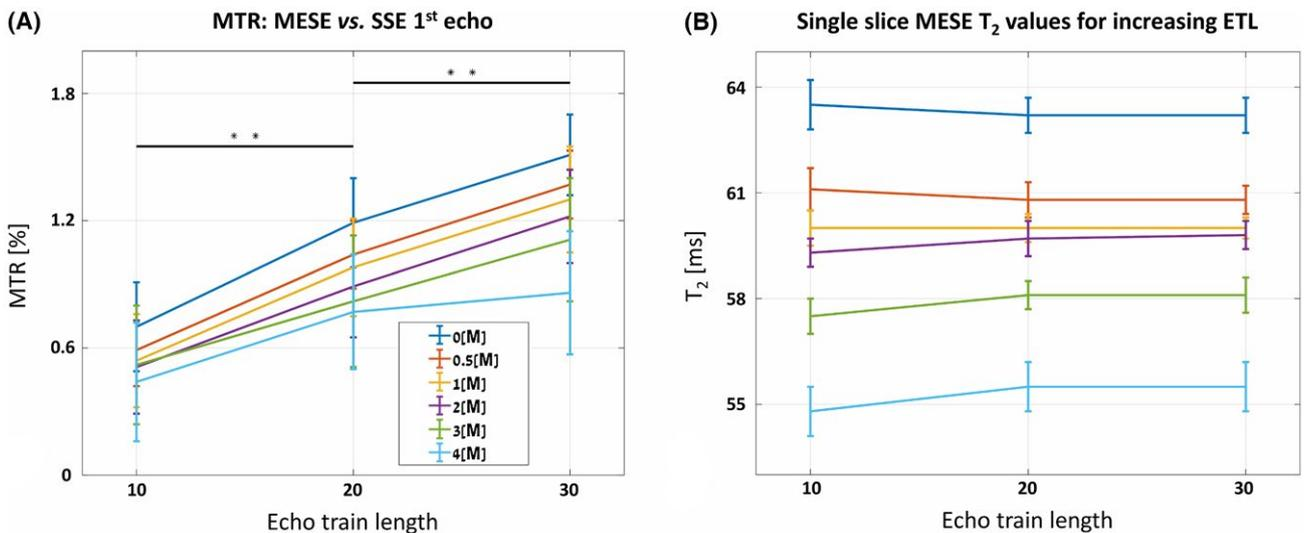
**FIGURE 3** MTR and  $T_2$  dependence on the ETL in a single-slice MESE scan of the urea phantom. (A) MTR between the 1st echo of SSE and MESE increases with longer ETLs (\*\* $P < 0.0001$ ). (B)  $T_2$  values remain stable for increasing ETLs, indicating that uniform MT attenuation occurs across the entire MESE echo train. Error bars represent SD within the ROI marked in Figure 1A
